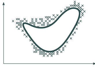
Curved line is the border of training space. The area enclosed in the curved line is the training space. × are artificial anomalies (more at sparse regions).
